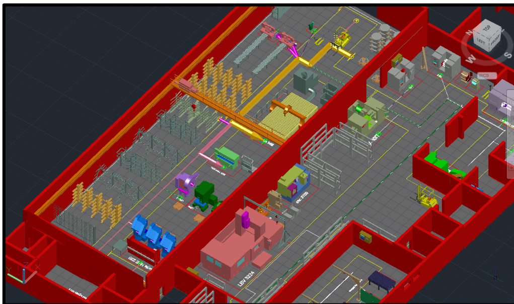
Figure 10. Sankey diagram in 3D layout of production system with logistics areas and tracks
