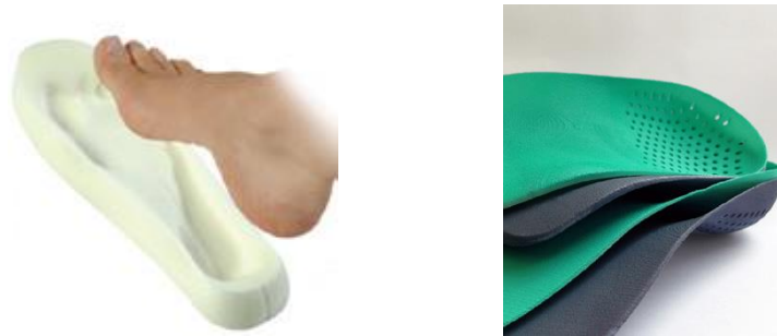
Figure 10. Foam scanning in traditional way and 3D printed insoles in modern way [5]
