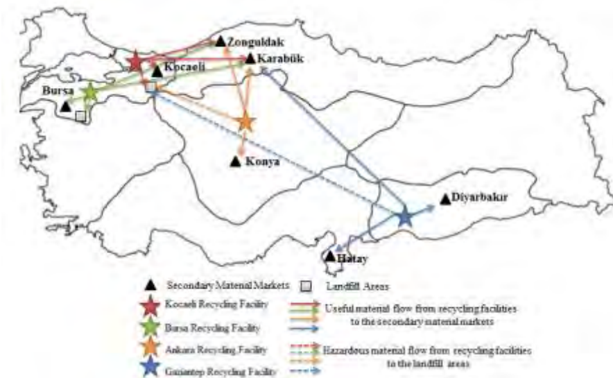
Figure 3. The Network Flow from Recycling Facilities to the Secondary Material Markets and Landfill Areas for Scenario 1
