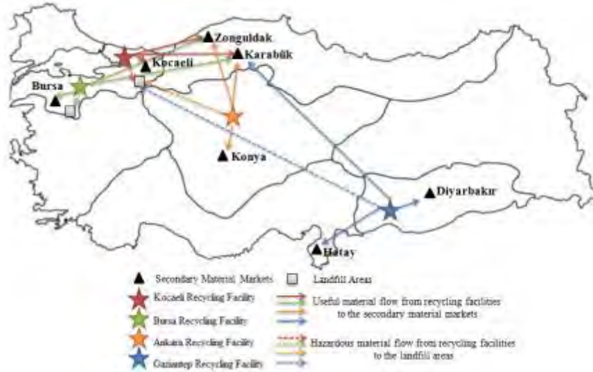
Figure 6. The Network Flow from Recycling Facilities to the Secondary Material Markets and Landfill Areas for Scenario 2
