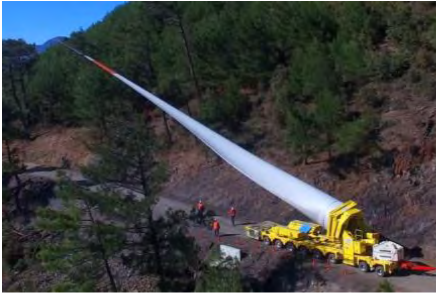
Figure 4. Scheuerle Blade Adapter for Turbine Blade Transportation
